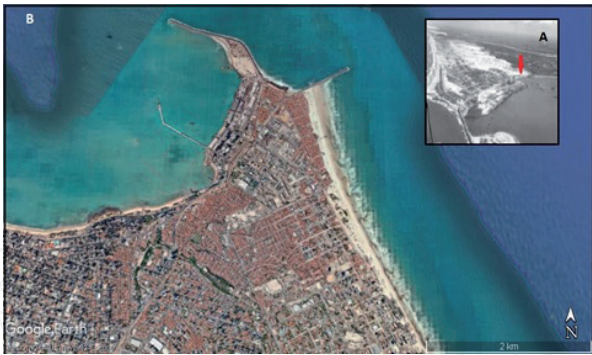
Figure 5. (A). East coast of Fortaleza city and Mucuripe harbor vicinity, with large dunefields. The red arrow shows the area where the bypass of dunes still took place after the construction of the harbor. (B). Complete urbanization of the dunefields, with cessation of dunes bypass.
