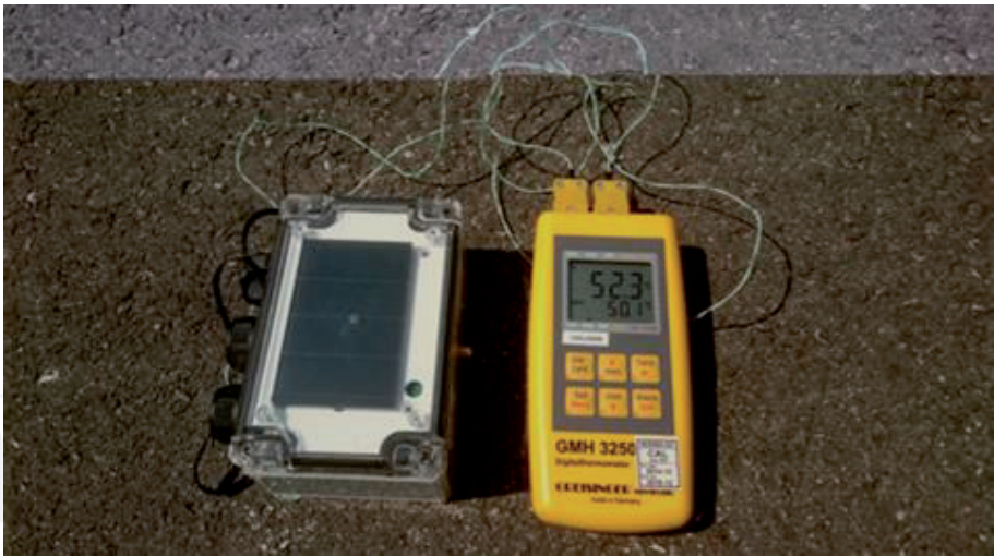
Figure 6. Measuring temperature inside the EnOcean low power, energy harvesting sensor module housing. The two channels of the thermometer (yellow device) are measuring the temperature of the solar cell (52.3°C) and supercapacitor (50.1°C), respectively. The outside temperature was 30°C.
