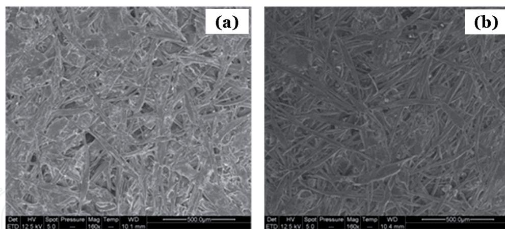
**Figure 3.** SEM images [magnification  $\times 500 \mu\text{m}$ ] of surface morphologies of papers made from soda-HP pulp (a) and paper made from soda-AQ pulp (b) (the encircled zones show the presence of fine elements).
