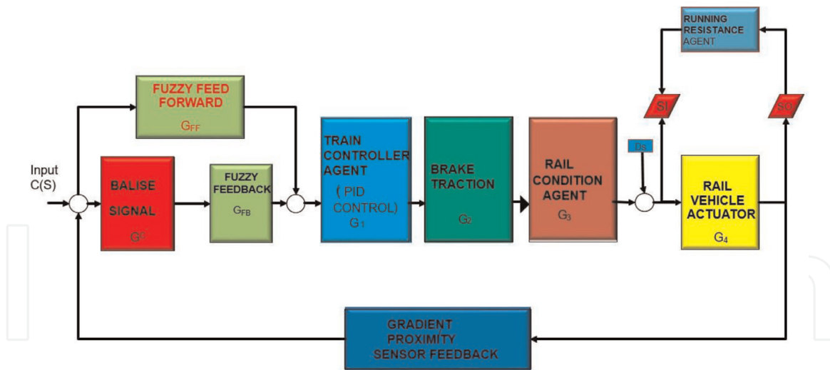
Figure 2. Fuzzy-PID controller implementation design for train controller agent.
