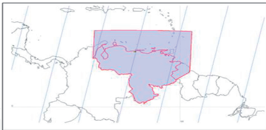
Figure 5. Remote Sensing Satellite-2 high-resolution camera (HRC) potential view capacity with field of view at +29^\circ .
