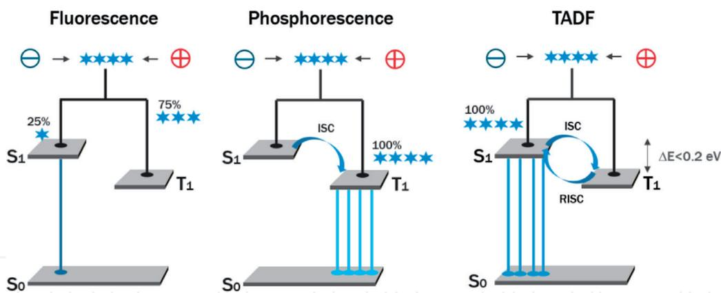
**Figure 1.** Schematic energy diagrams of fluorescent, phosphorescent, and TADF molecules and their corresponding excitation and de-excitation pathways, when used in OLEDs. Fluorescence often relates to the first emitter material generation. Phosphorescence is the second material generation. TADF marks the latest conceptual development. Figure courtesy of CYNORA.
