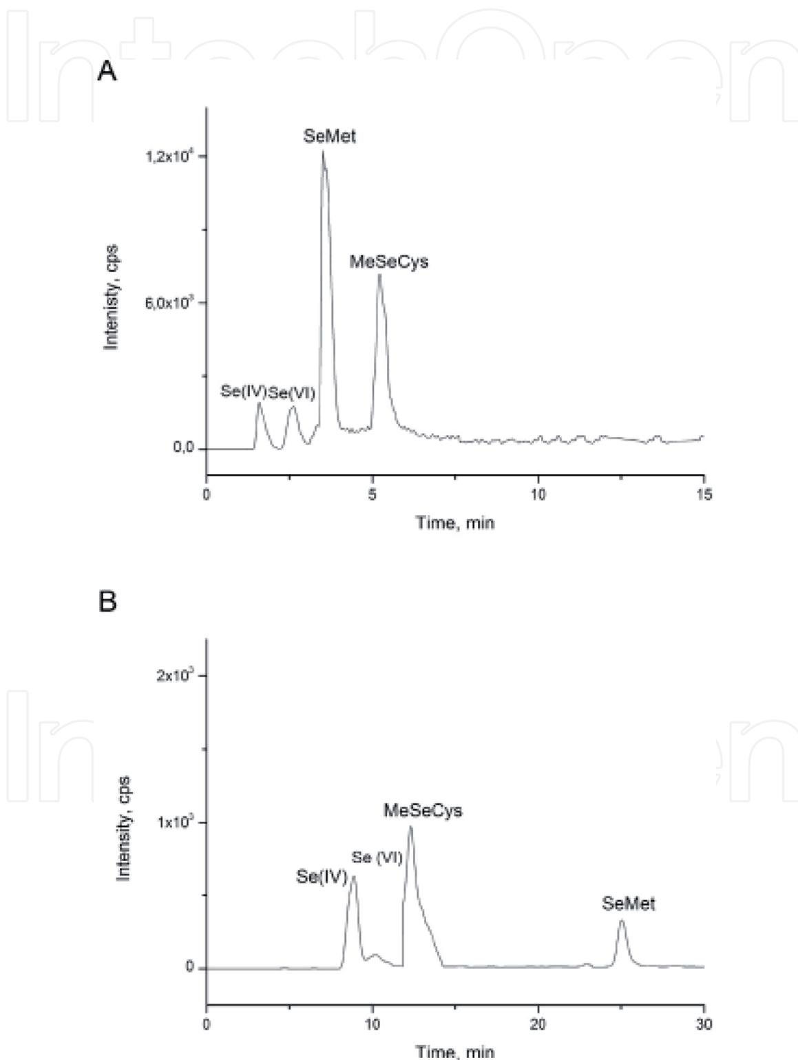
**Figure 2.** The chromatographic separation of selenium species present in onion leaf extracts in (A) HILIC mode and (B) RP mode. (A) Atlantis HILIC (silica) column, mobile phase: 85% MeOH and 8 mM CH<sub>3</sub>COONH<sub>4</sub>, pH 7. (B) Luna C8 column, mobile phase: 99.5% HCOOH and 0.5% ACN [79]. Reprinted with permission from Elsevier.
