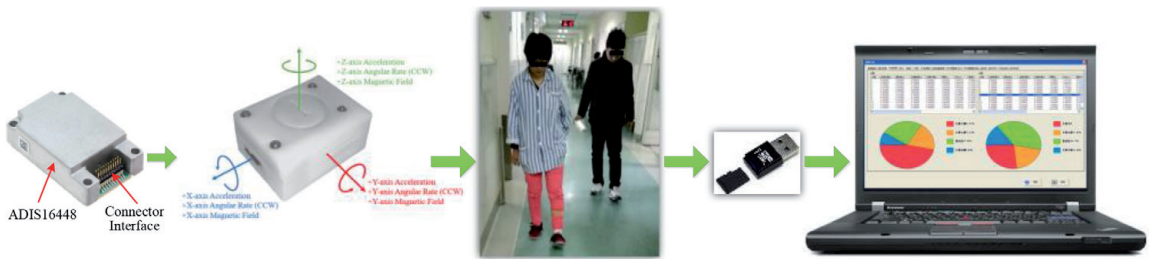
Figure 11. ADIS16448 iSensor ® device used for gait data collection.
