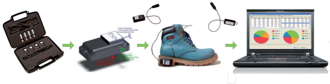
Figure 9. MEMSense nIMU used for gait data collection.
