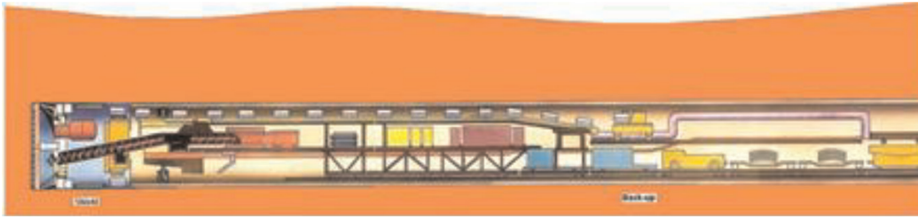
Figure 1. Schematic view of a TBM.
