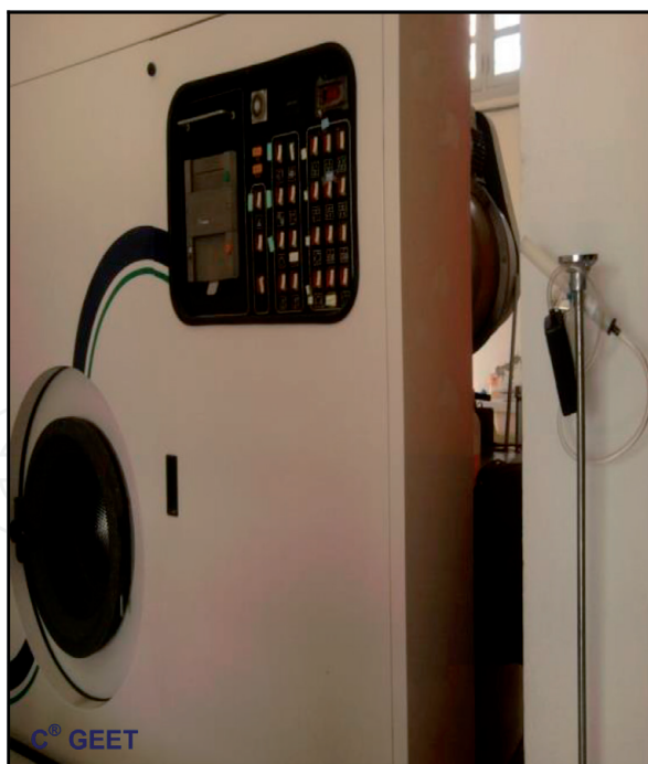
Figure 1. Active air monitoring using fixed sampling station.
