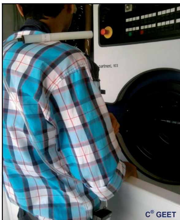
Figure 2. Active air monitoring using personal sampling.
