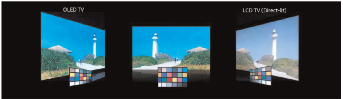
Figure 18. Picture quality change at the off-axis of the OLED TV and the LCD TVs.
