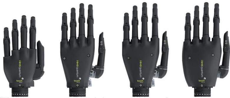
Figure 6. i-Limb Quantum by Touch Bionics, from left to right: extra small, small, medium, and large.
