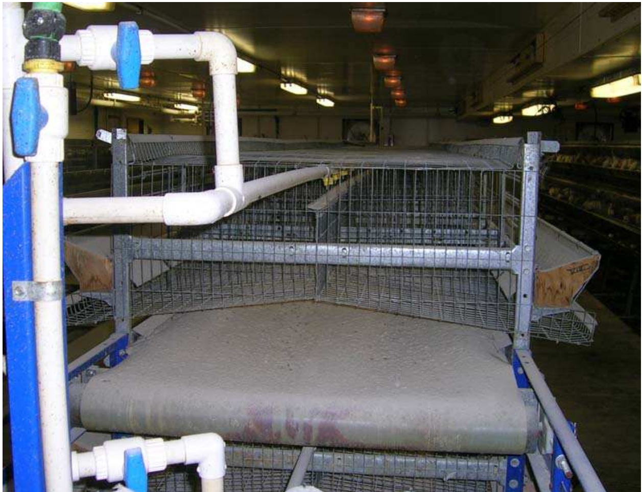
Fig. 3. Cage over manure conveyer belt.
