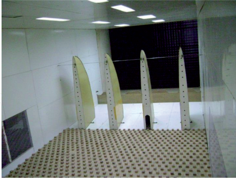
Figure 4. Couinean vortex generators, barrier, and roughness elements of the full-depth boundary layer simulation.
