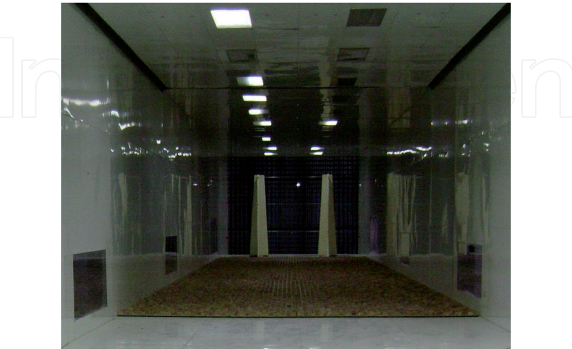
Figure 7. Irwin vortex generators and roughness elements of the part-depth boundary layer simulation.
