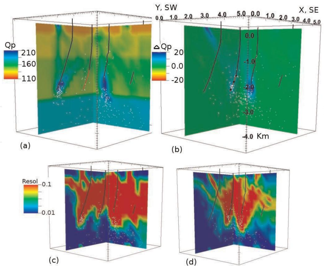
**Figure 5.** (a) Qp tomography results for period 1 along cross sections AA' and BB' shown in Figure 1b; (b) results for  $\Delta Q_p$  for period 2, Qp scale on left; (c) resolution for period 1; (d) resolution for period 2. Resolution scale is for diagonal of resolution matrix, where red is greater than 0.1 and blue is less than 0.01.
