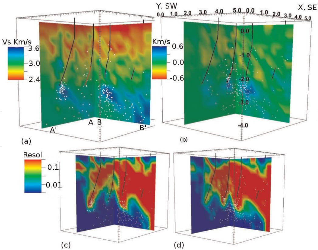
**Figure 4.** (a) Vs tomography results for period 1 along cross sections AA' and BB' shown in Figure 1b; (b) changes in Vs results for period 2, i.e.,  $\Delta V_s$ ; (c) resolution for period 1; (d) resolution for period 2.
