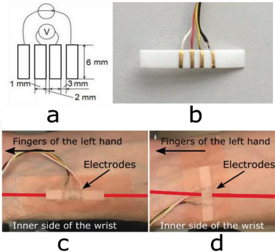
**Figure 8.** Dimensions (a), design (b), and placement of a custom-made flexible four-electrode system in the case of a distal (c) and circular (d) locations on the wrist, where the thick red line denotes the approximate location of the radial artery (reprinted from [27]).
