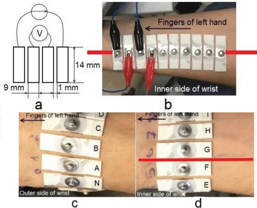
**Figure 10.** Modified dimensions of the standard ECG electrodes in utilised four-electrode system (a) and the placement on the wrist in distal (b) and circular configuration (c and d), where the thick red line denotes the approximate location of the radial artery (reprinted from [27]).
