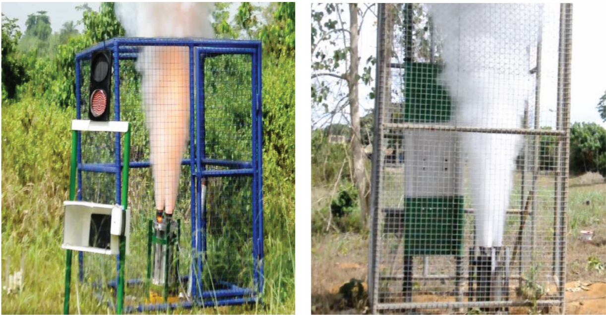
Figure 8. Static test rigs with tri-cluster rocket motors.
