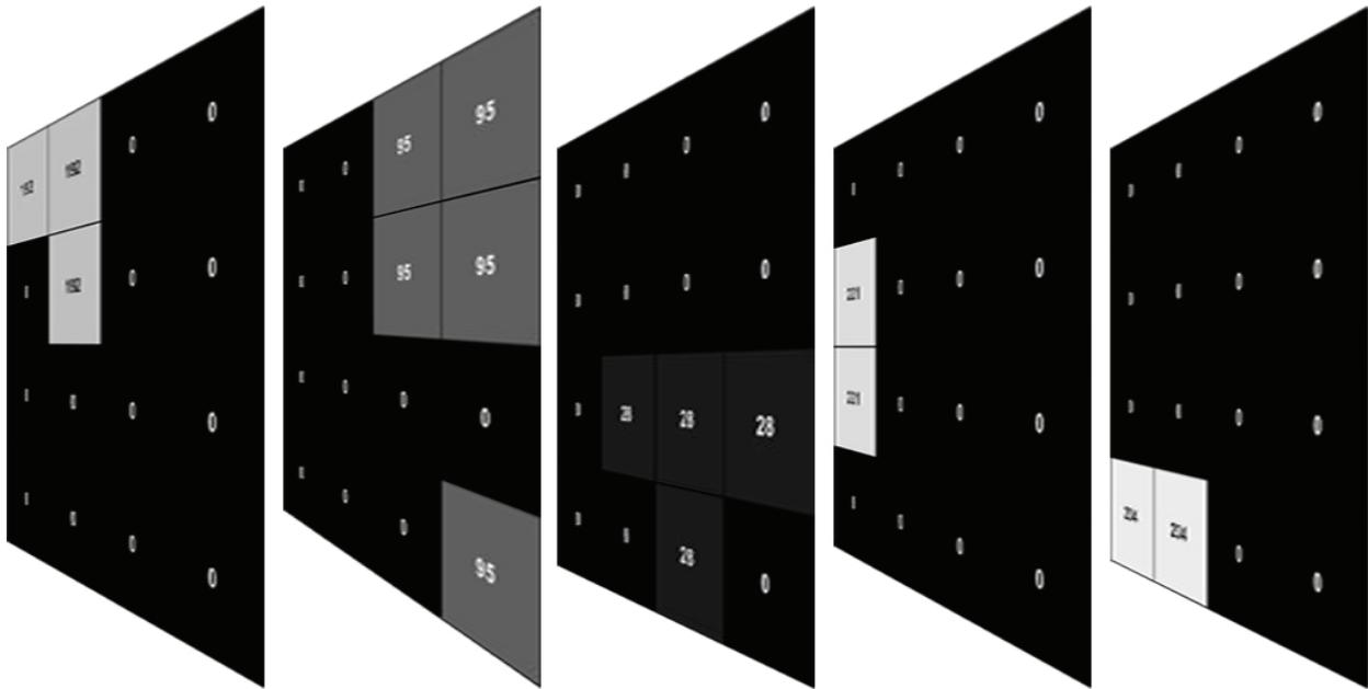
Fig. 2. Image Slice Representation of the image of Fig.1: 1<sup>st</sup> image slice of 192 intensity, 2<sup>nd</sup> image slice of 95 intensity, 3<sup>rd</sup> image slice of 28 intensity, 4<sup>th</sup> image slice of 221 intensity and 5<sup>th</sup> image slice of 234 intensity.
