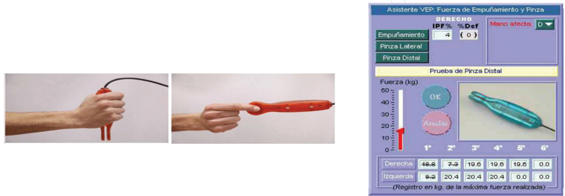
Figure 4. PC-based hand dynamometer used (probe detail).
