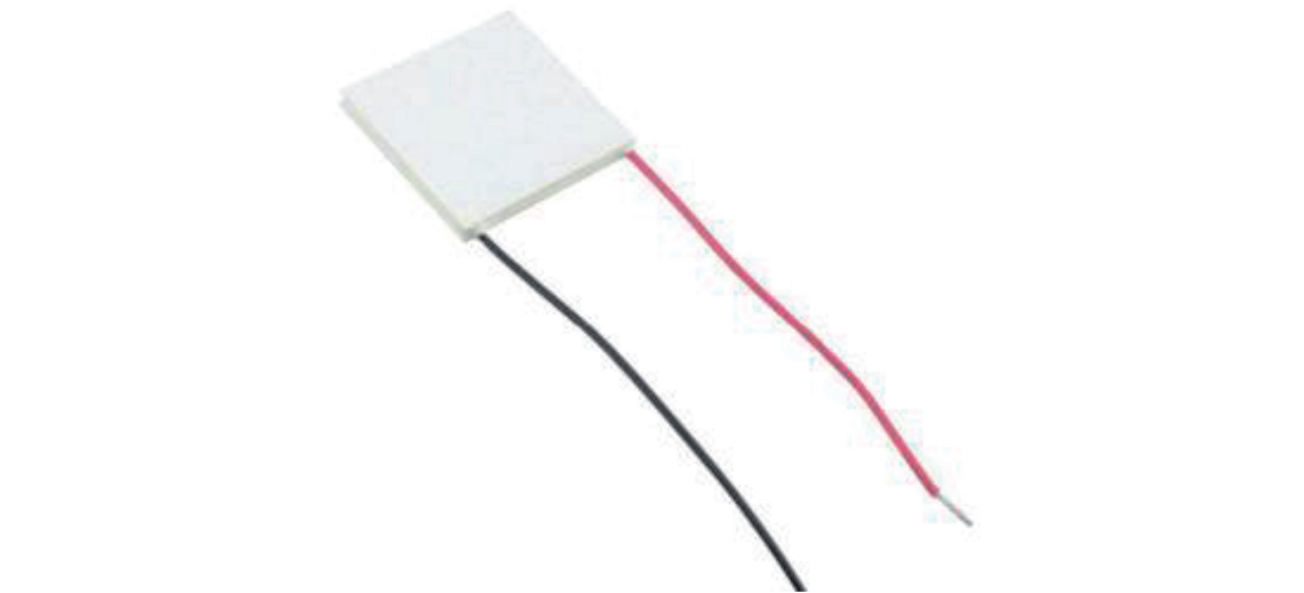
Figure 6. The special silicon junction of the Peltier device can provide a voltage potential that provides a current flow that creates a cooling effect on one side of the device while creating a heating effect on the other side. Source: [1].
