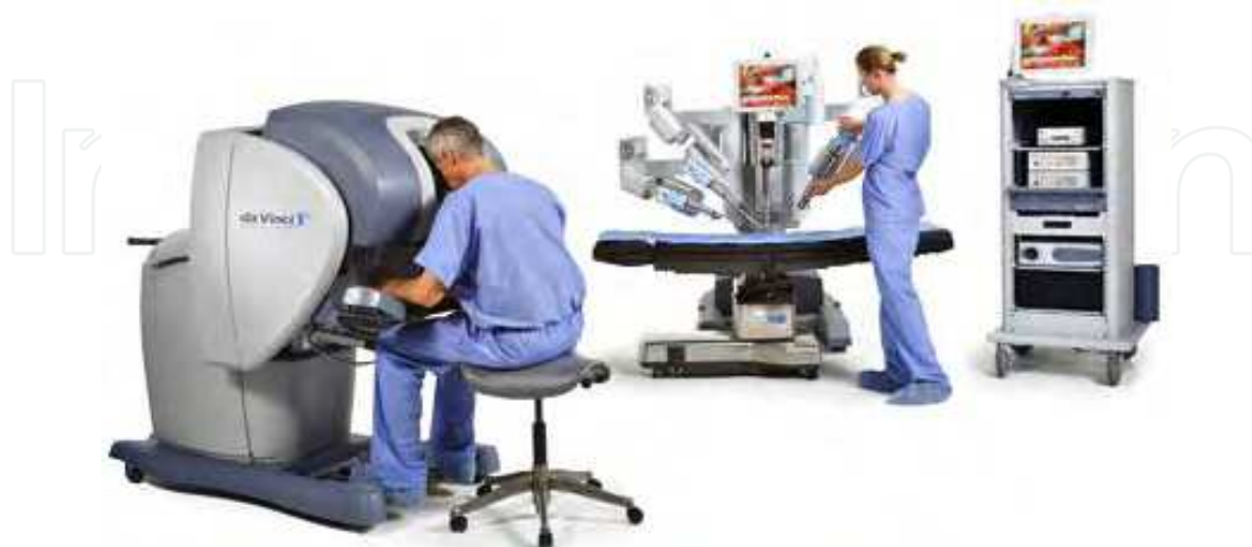
Figure 1. da Vinci system®. It consists of a surgeon's console, a patient-side cart with three or four interactive robotic arms, a high-performance InSite ® Vision System and proprietary EndoWrist ® Instruments
