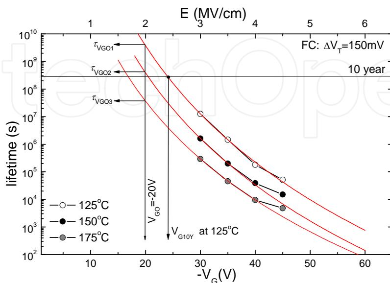
Fig. 13. Estimation of the lifetime and ten year operation voltage by power-law model.
