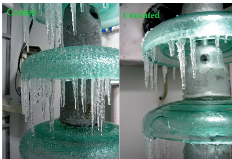
Figure 5. Comparison of the ice formation on the uncoated and superhydrophobic-coated insulators [5].
