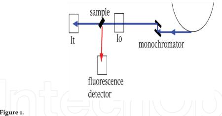
Figure 1. XAS instrumentation.
