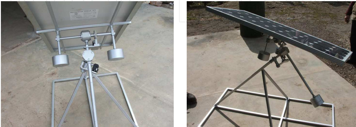
Fig. 20. The physical prototype of the polar tracking system
