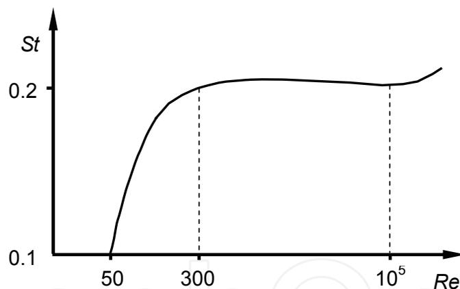
Fig. 5. *Strouhal* number as a function of *Reynolds* number for flow around a cylindrical body
