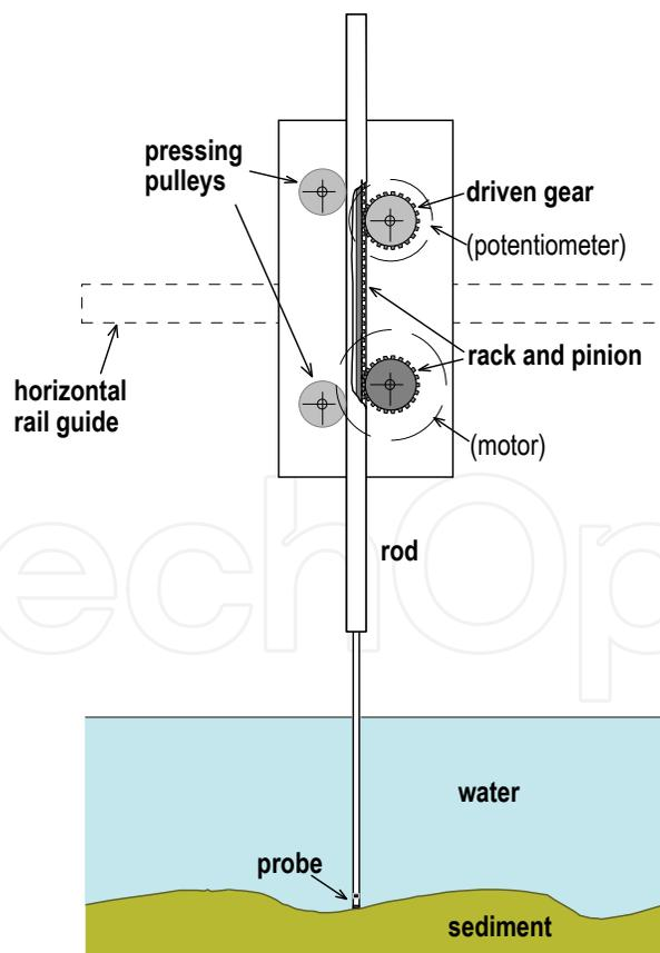
Fig. 7. Pictorial description of a complete mechanism for vertical motion of a bed profiler; the electric motor, the potentiometer and the pressing leaf spring are mounted on the back face; guide wheels are not shown.
