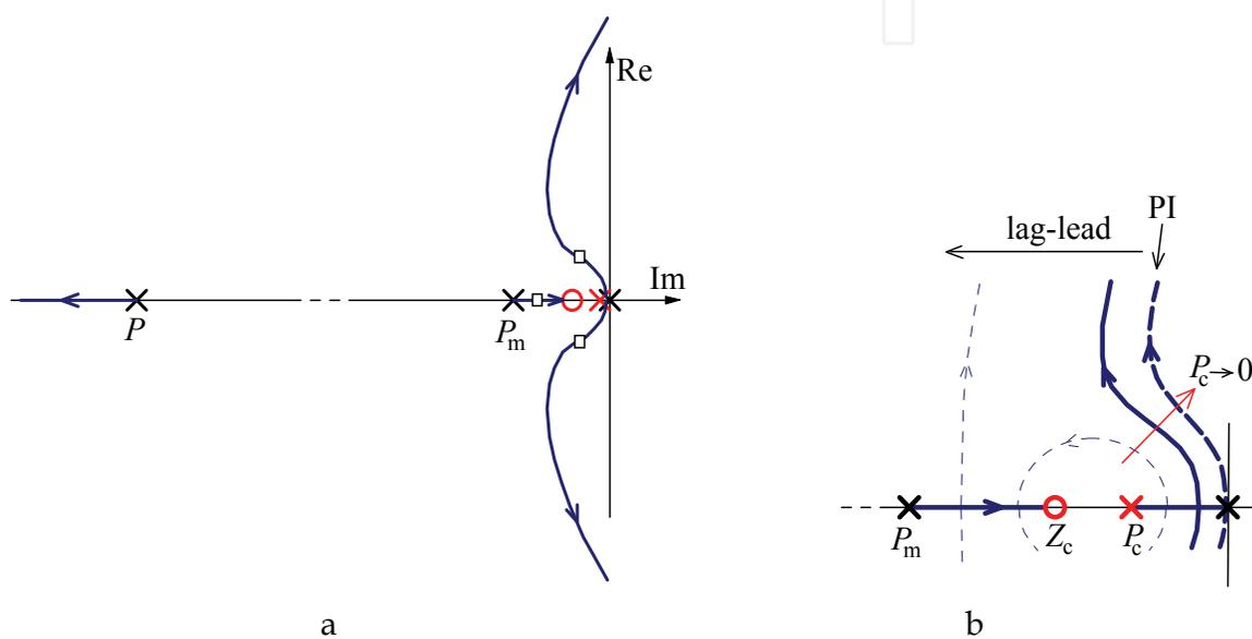
Fig. 12. Root locus sketch of the closed-loop system: a) general plan; b) enlarged view near the origin showing the effect of varying the controller pole  $P_c$  from lag-lead to PI.
