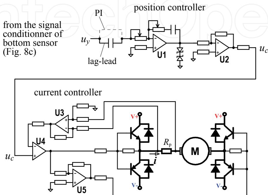
Fig. 11. Electronic power stage and controller circuit schematics.
