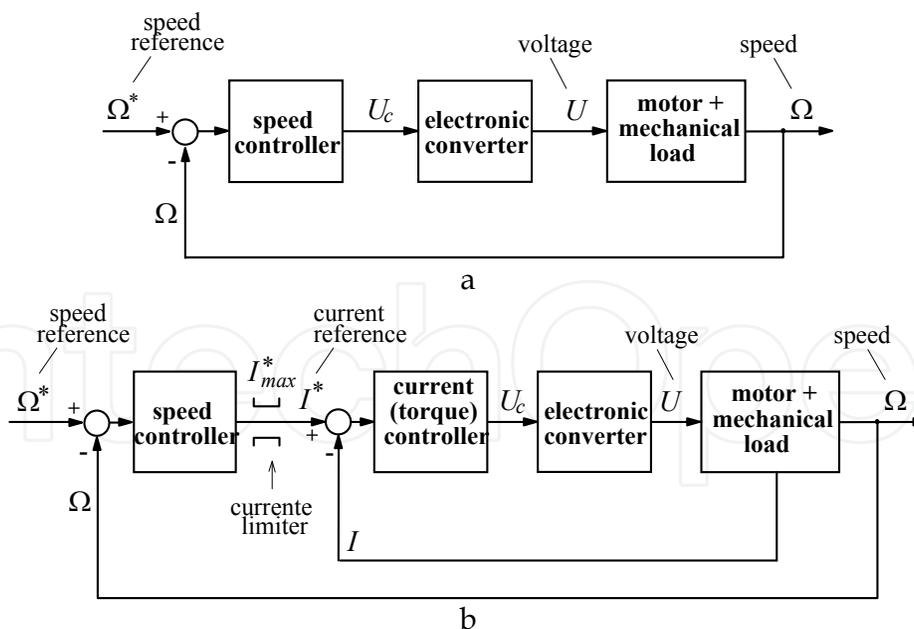
Fig. 9. Closed loop dc motor speed drive methods: a) with direct voltage adjustment; b) with a subordinate current control loop.
