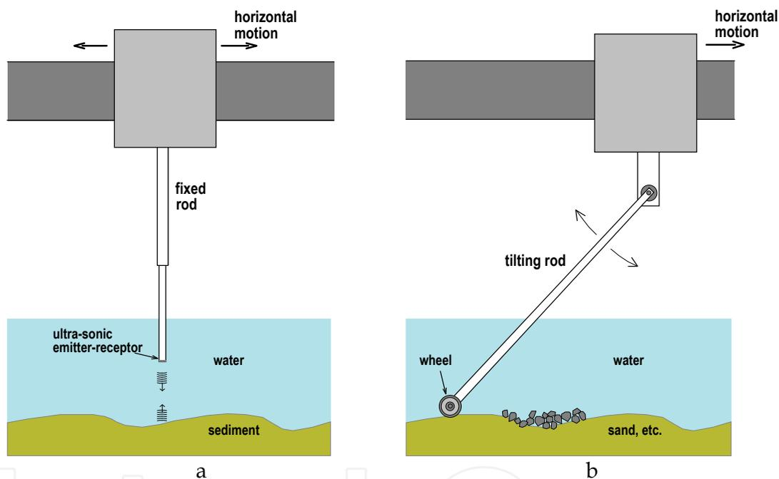
Fig. 2. Other bed profiling solutions: a) ultrasonic transit time; b) trolley with tilting rod.
