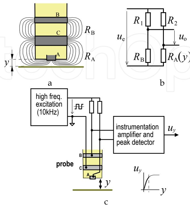
Fig. 8. a) Details of the bottom proximity sensor probe showing the fields of currents between electrodes; b) Bridge circuit for transducing the distance  $y$  to the bottom; c) block diagram showing excitation and signal conditioning stages.
