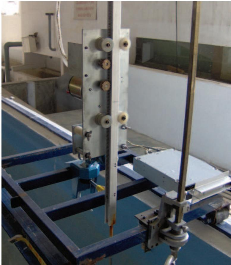
Fig. 13. Photograph showing the instrument block in a chariot over the flume.
