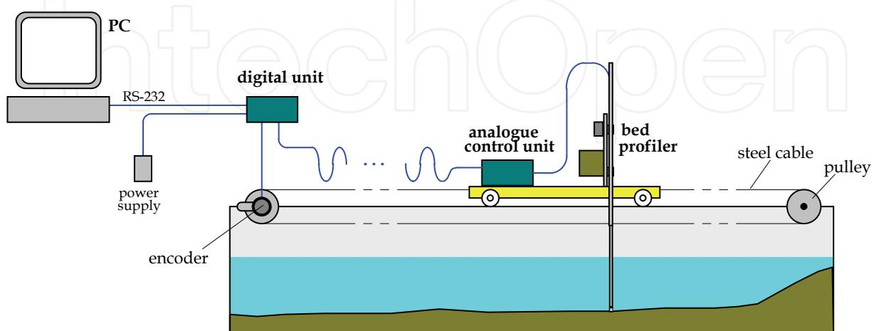
Fig. 14. Synoptic sketch of the bed profiler and the data acquisition system used in the flume model
