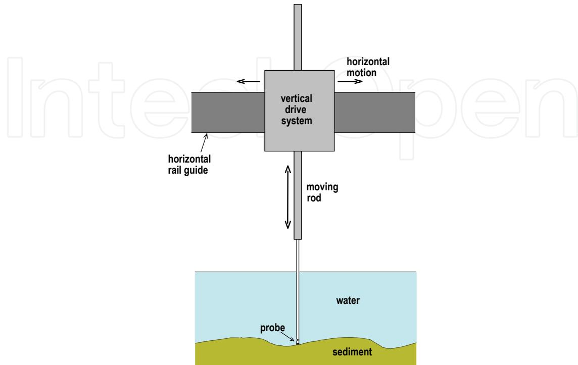
Fig. 1. Conceptual principle of a servo driven bottom follower.
