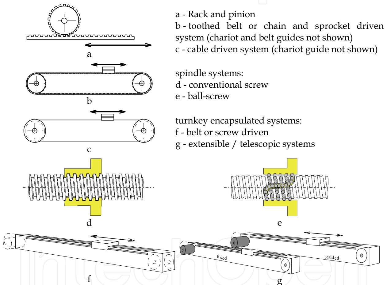
Fig. 3. Typical solutions for horizontal movement of bed profiling devices
