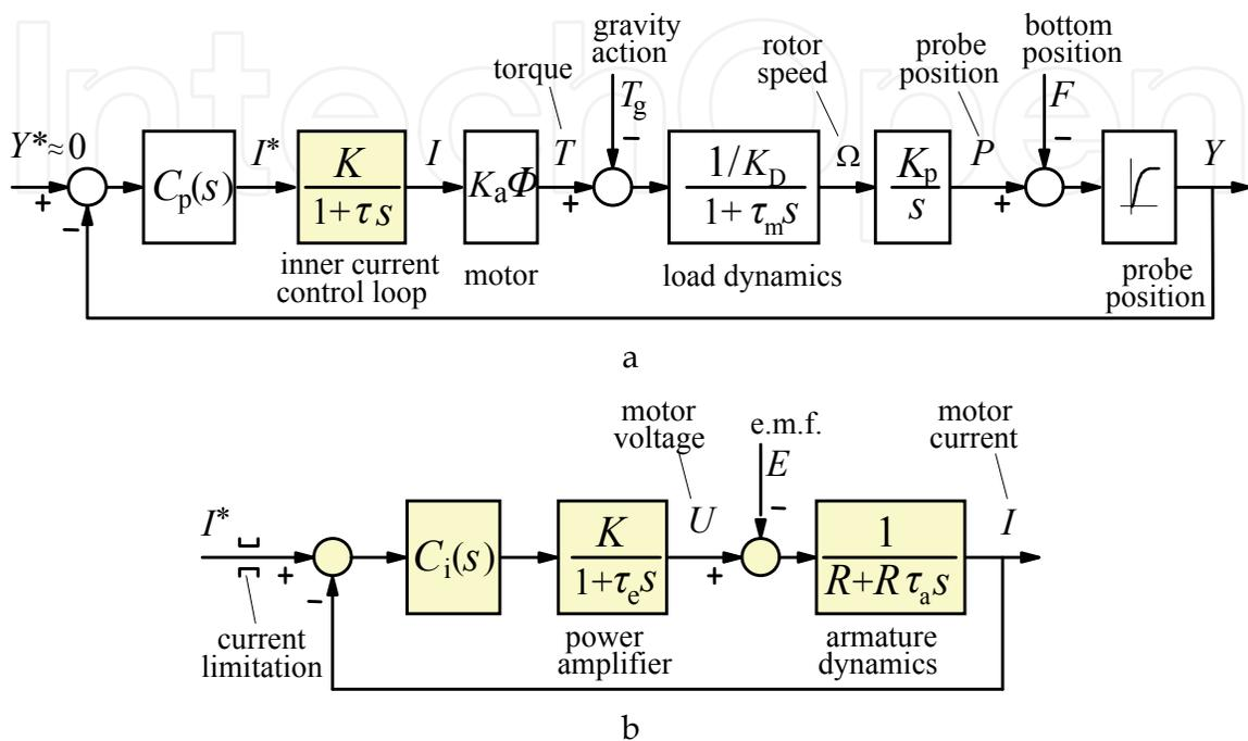
Fig. 10. a) Block diagram of the bottom tracking system. b) Detail of the inner current control loop.
