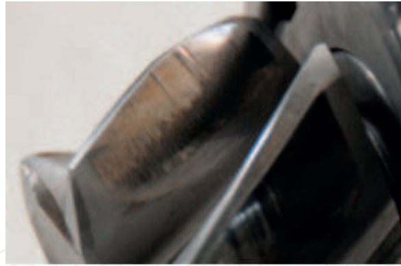
Figure 6. Scuffed area on the tooth flank of a spiral bevel gear.
