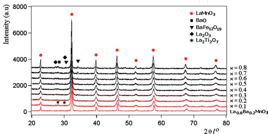
**Figure 8.** X-ray diffraction pattern of  $La_{0.8}Ba_{0.2}Fe_xMn_{1/2(1-x)}Ti_{1/2(1-x)}O_3$  ( $x = 0.1-0.8$ ) [22].
