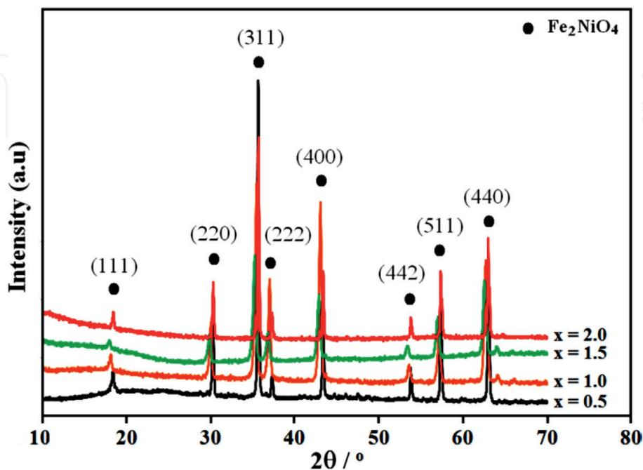
**Figure 11.** X-ray diffraction patterns of  $\text{Ni}_x\text{Fe}_{3-x}\text{O}_4$  of ( $x = 0.5\text{--}2.0$ ) [25].
