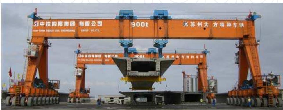
Fig. 1. Hoisting-girder transporter with 900T load
