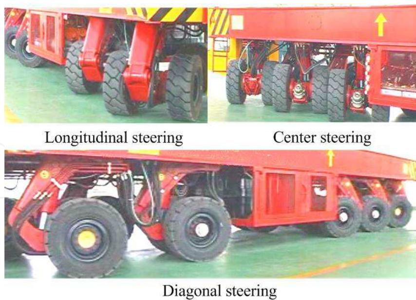
Fig. 18. Test of multimode steering
