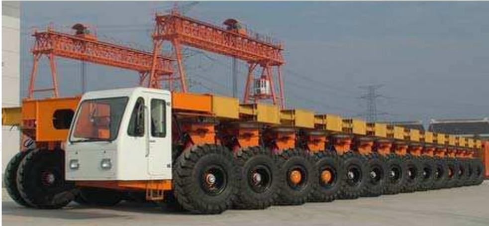
Fig. 2. DCY900 powered transportation vehicle
