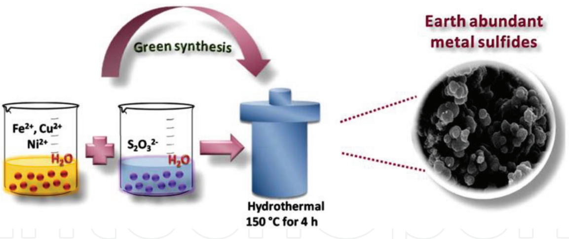
Figure 1. Schematic illustration of the hydrothermal synthesis of \text{FeS}_2 , \text{CuS} , and \text{NiS}_2 powders. Reproduced with permission from [10].
