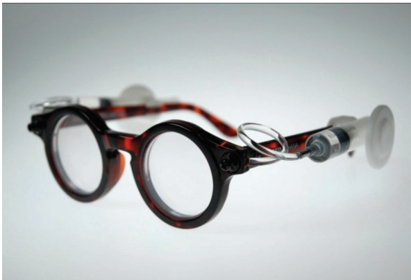
Figure 4. Adspecs glasses can quickly adjust refractive power based on the amount of silicone solution injected into the spectacles.
