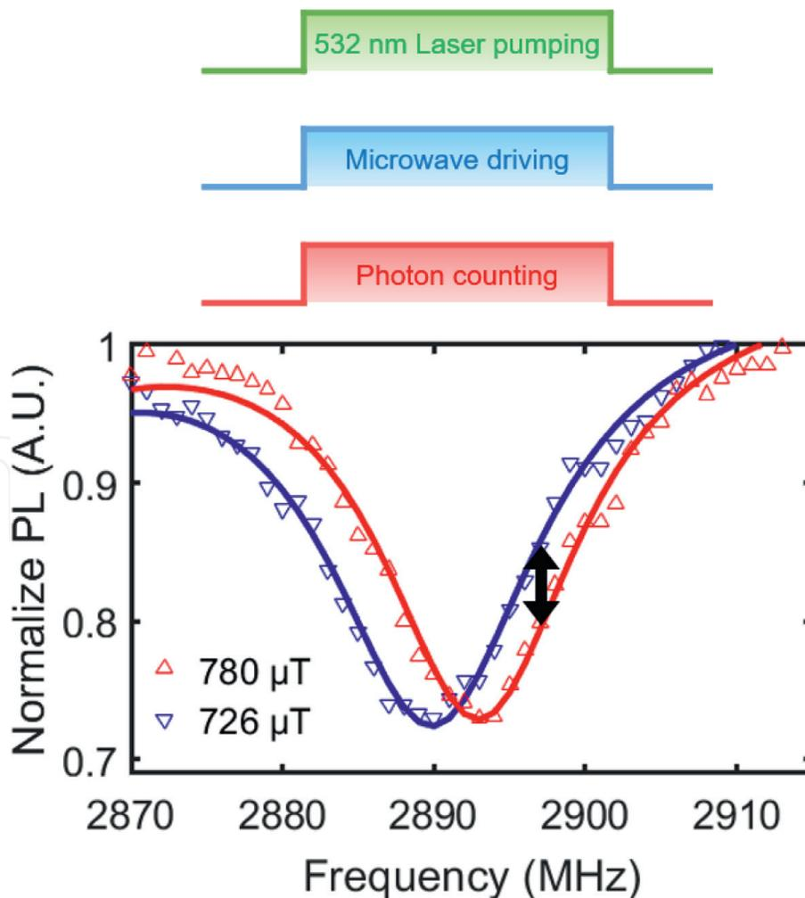
**Figure 4.** Sensing dc magnetic field based on CW-ESR measurement. Continuous wave of laser and microwave photons are used. The shift in frequency gives an information about the magnitude and direction of external magnetic field.
