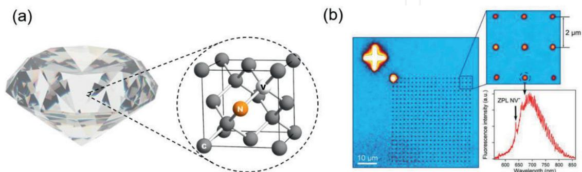
**Figure 2.** Physical properties of diamond NV center. (a) Crystal structure of NV center in a diamond lattice. NV center consists of nitrogen substitutional defect and carbon vacancy. (b) Precise formation of NV centers using focused ion beam (FIB) implantation of nitrogen. Reprint with permission from [27]. Copyright (2013) Wiley-VCH Verlag GmbH & Co. KGaA. Reproduced with permission.
