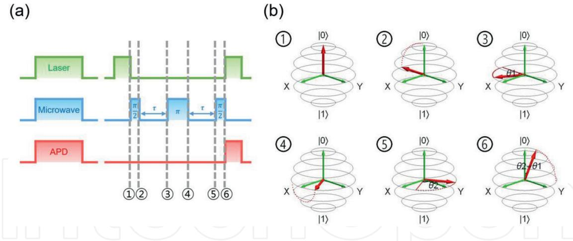
**Figure 7.** Sensing ac magnetic field based on spin Hahn echo measurement. (a) Schematics of the Hahn echo pulses. (b) Bloch representations of the spin status according to the numbers indicated in (a).
