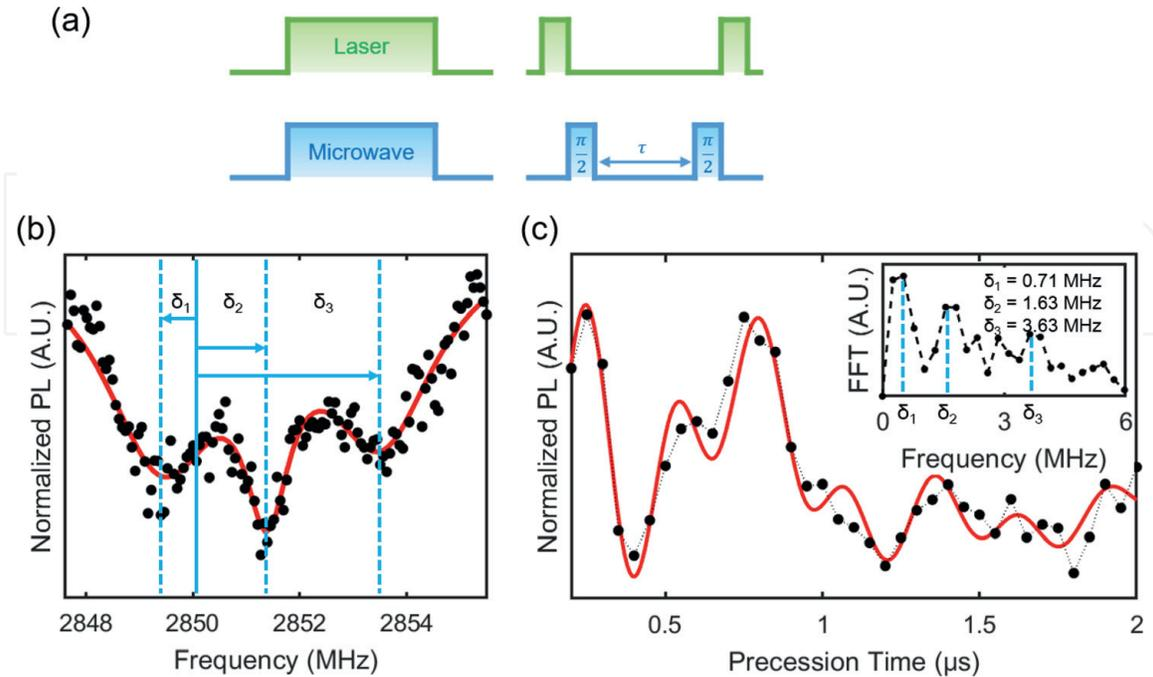
**Figure 5.** Sensing dc magnetic field based on Ramsey interferometry. (a) Schematics of laser and microwave pulse used for the measurement. (b) A close view of the resonance peak in CW-ESR reveals three sub-features resulting from the NV's hyperfine coupling with  $^{14}\text{N}$  nuclear spin. (c) Ramsey measurement with the detunings in (b) shows the beatings of three oscillations. Subset presents the FFT of the Ramsey signal showing three peaks corresponding to the detunings.
