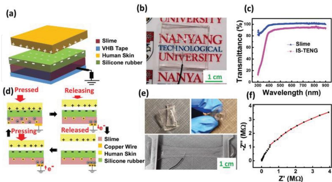
**Figure 3.** (a) Schematic diagram of the IS-TENG. (b) Digital photo of the highly transparent IS-TENG. (c) Transmittance spectra of the slime (ionic conductor) and the IS-TENG with respect to a glass slide. (d) Schematic illustration of the working mechanism of the IS-TENG. (e) Digital photos of the IS-TENG under various mechanically deformed states such as axial strain up to 700%, rolled, and folded. (f) EIS measurement of the slime (ionic conductor) [57].
