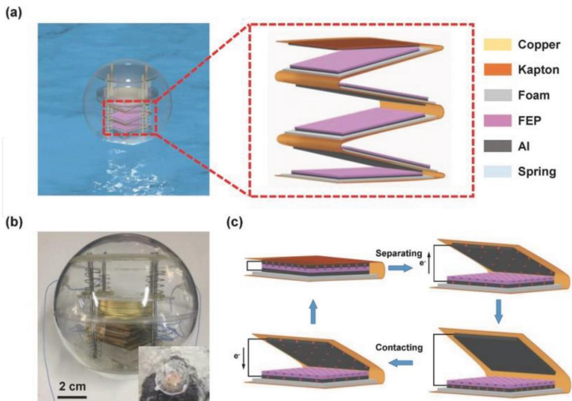
**Figure 10.** (a) Schematic diagram of the spherical TENG with spring-assisted multilayered structure floating on water, and schematic representation enlarged structure for the zigzag multilayered TENG with five basic units. (b) Photographs of the as-fabricated TENG device. (c) Working principle of each TENG unit of the spherical TENG [97].
