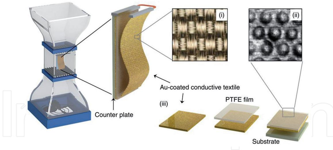
**Figure 12.** Schematic diagrams of a wind tunnel and the structural design of a flutter-driven triboelectric generator including surface characteristics of (i) a highly flexible flag, (ii) a counter plate, and (iii) the fabrication of the counter plate [106].
