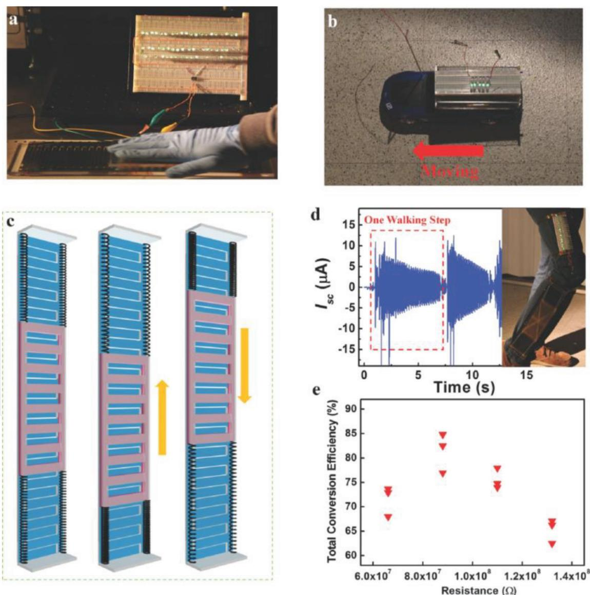
**Figure 4.** Applications of GF-TENG for harvesting a wide range of mechanical energy. (a) Harvesting energy from sliding of a human hand. (b) Harvesting energy from acceleration or deceleration of a remote control car. (c) Device structure for noncontact GF-TENG. (d) Harvesting energy from people walking by noncontact GF-TENG and the real-time measurement of  $I_{sc}$ . (e) Total conversion efficiency of noncontact GF-TENG for harvesting slight vibration under different load resistances [59].
