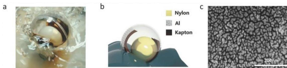
**Figure 9.** Device structure, basic operations of the freestanding-triboelectric-layer-based nanogenerator (RF-TENG) with a rolling Nylon ball enclosed. (a) Photograph of a rocking nanogenerator floating on water. (b) Schematic diagrams of freestanding-structured design. (c) SEM image of nanorod structure on the Kapton surface [93].
