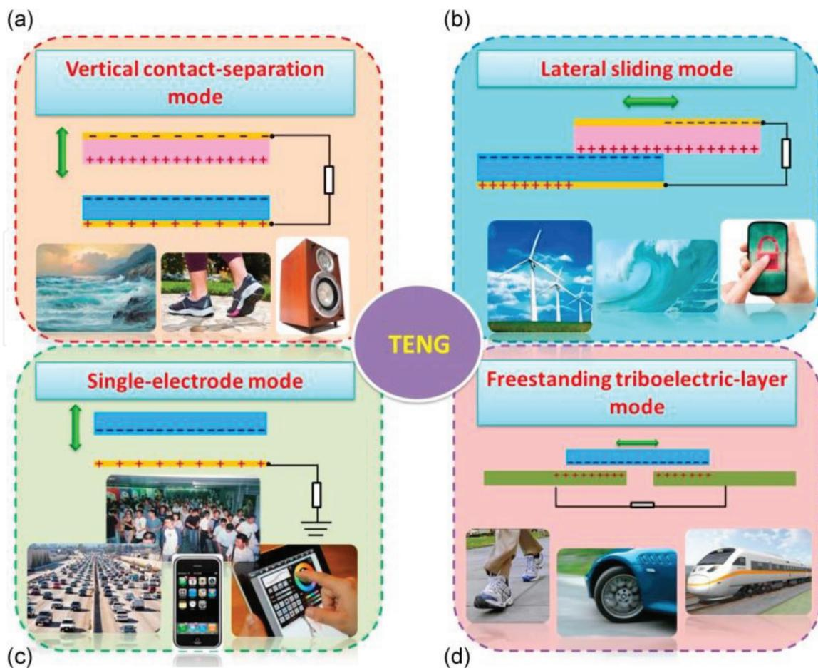
**Figure 1.** The four fundamental modes of triboelectric nanogenerators: (a) vertical contact separation mode, (b) in-plane contact-sliding mode, (c) single-electrode mode, and (d) freestanding triboelectric-layer mode [9].
