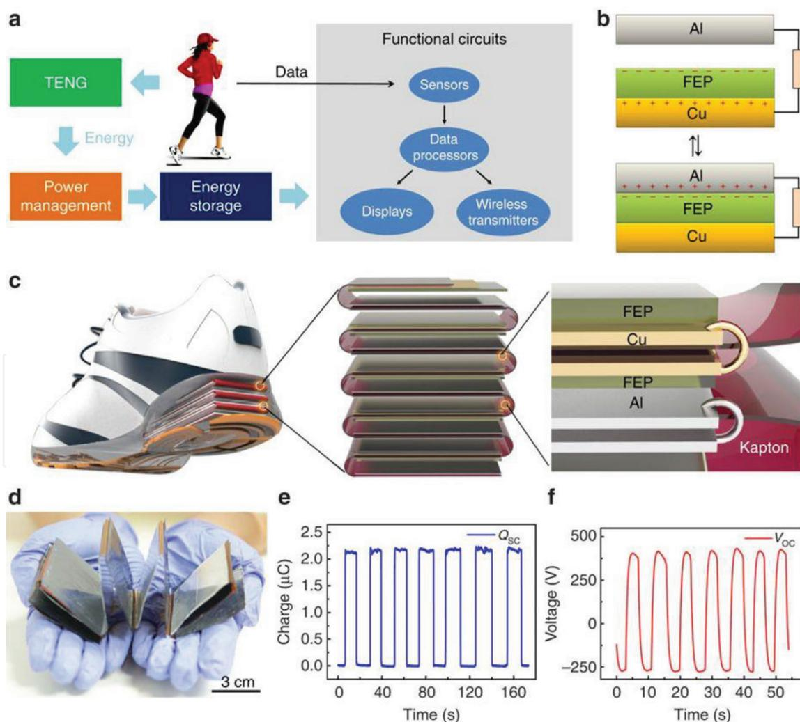
**Figure 2.** (a) System diagram of a TENG-based self-powered system, (b) working mechanism of an attached-electrode contact-mode TENG, (c) structure of the designed multilayer TENG, (d) photo of an as-fabricated TENG, (e) triboelectric charge output, and (f)  $V_{oc}$  output of the as-fabricated TENG [14].
