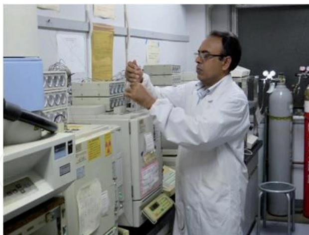
Figure 4. Injecting air samples into GC for determination of \text{CH}_4 and \text{N}_2\text{O} concentrations.
