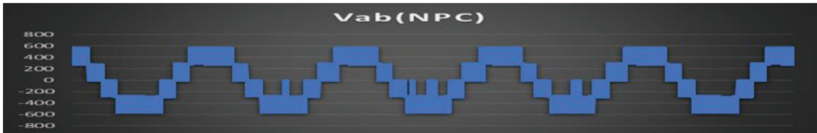
Figure 8. Output voltage of NPC Inverter.
