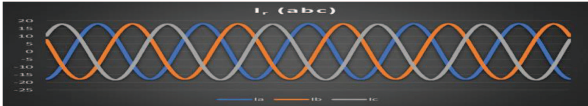
Figure 7. Simulation result rotor side converter current.
