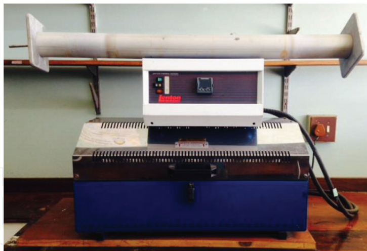
Figure 4. Image of the split tube furnace and aluminum reactor used in the fabrication of ZnO nanostructures.
