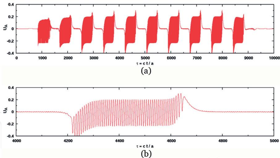
**Figure 5.** (a) Train of the EHF pulses and (b) the shape of a single pulse generated by the circuit with  $d = 200$  at the oscillation period  $T \approx 8$  when switching the bias voltage up to  $e_B = 2.0$  at the rise-time  $T_R \approx 400$  ([20]; licensed under a creative commons attribution (CC BY) license).
