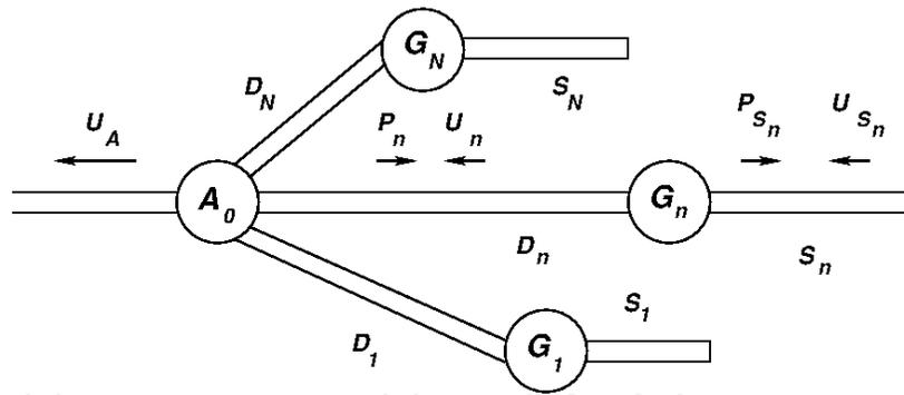
**Figure 6.** Schematics of a parallel connection of active circuits where, in distinction from [21], different lengths of all microstrip sections  $D_n$  and stubs  $S_n$  are assumed as needed for quasi-chaotic oscillations.
