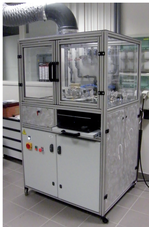
Figure 6. Close-proximity SALD approaches. Left: Schemes of the initial SALD systems reported by Kodak. Right: system developed at the LMGP.
