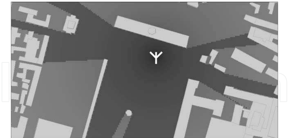
Fig. 6. Top view of the discrete line-of-sight region (dark grey) with the source point in the center (white cross). Building interior is shown in light grey.
