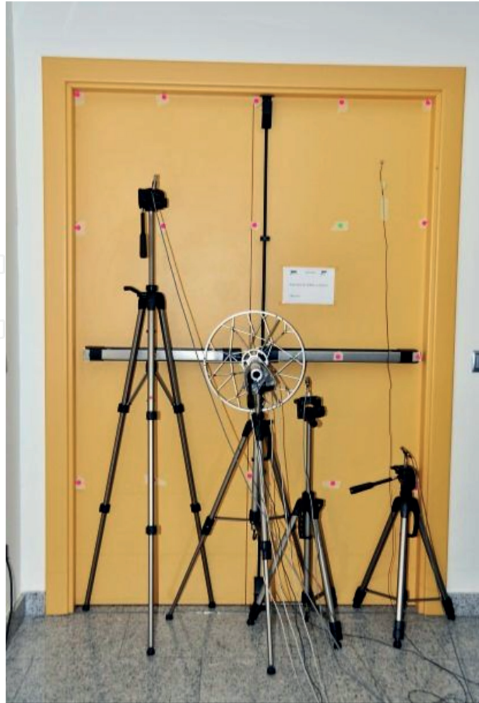
Figure 4. Example of the SONAH measurement layout.
