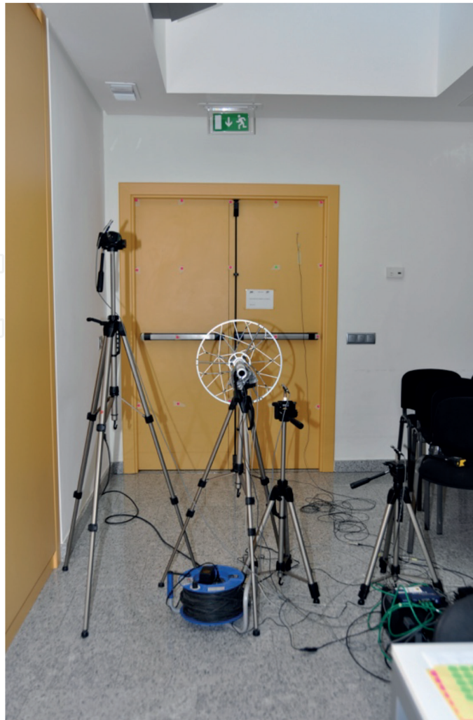
Figure 3. Example of the beamforming measurement layout.
