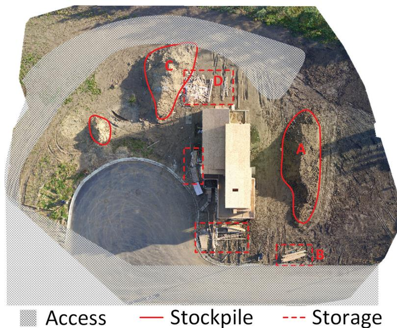
**Figure 4.** Qualitative constraints identification in GoogleEarthWork: geo-relationship between accesses, stockpiles, storage area, and the building identified from high-resolution panoramic images stitched from aerial photos.
