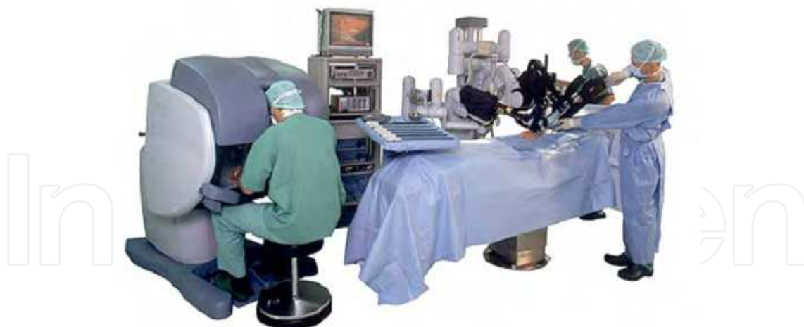
Figure 4. DaVinci robotic system by Intuitive Surgical Inc
