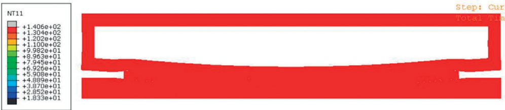
Figure 18. Nodal temperature results at t = 438 s (relative to current load step).
