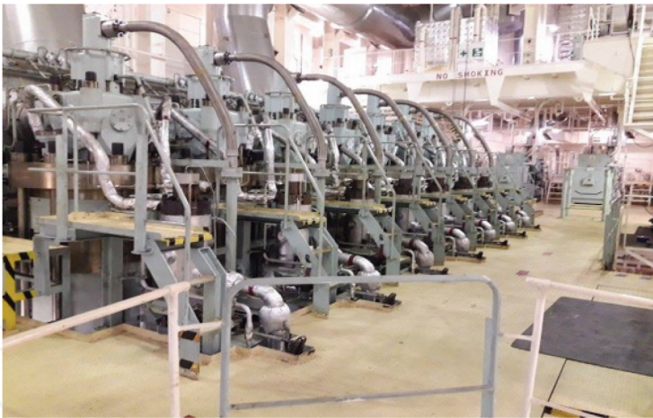
Figure 6. Main diesel engine (MAN B&W 7S80MC-C).
