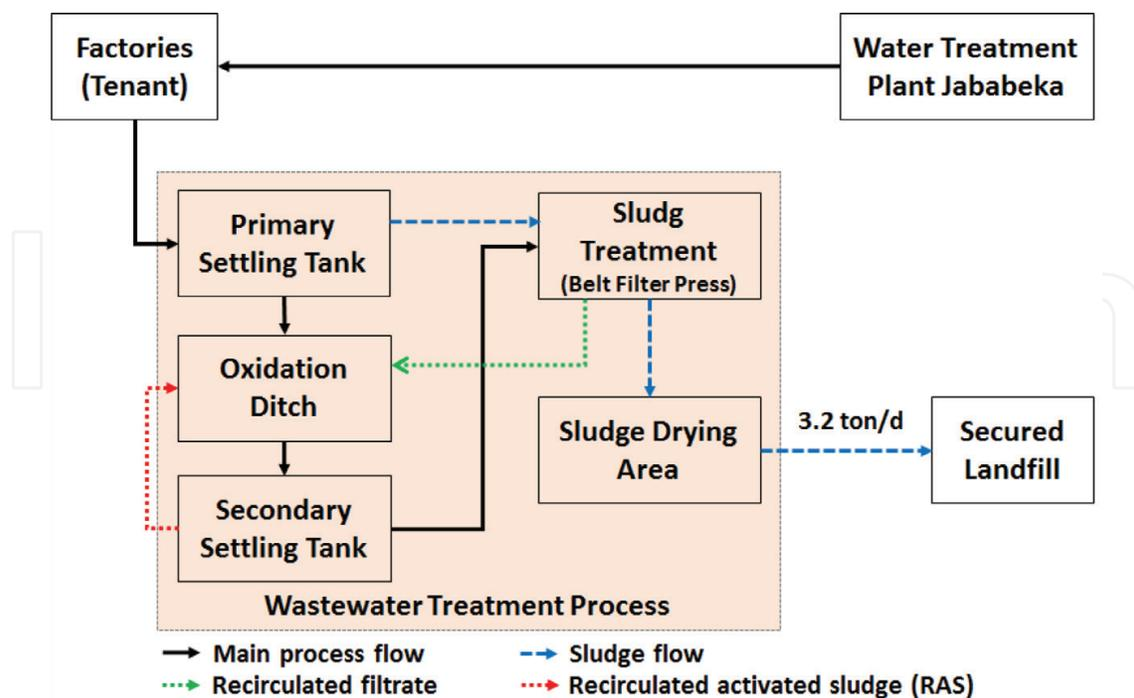
**Figure 1.** Schematic flow diagram of Jababeka's wastewater treatment facilities.
