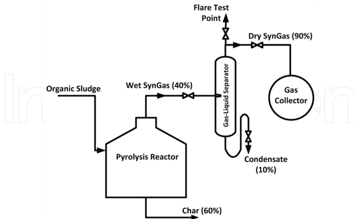
**Figure 5.** Simplified schematic diagram of organic sludge pyrolysis process.
