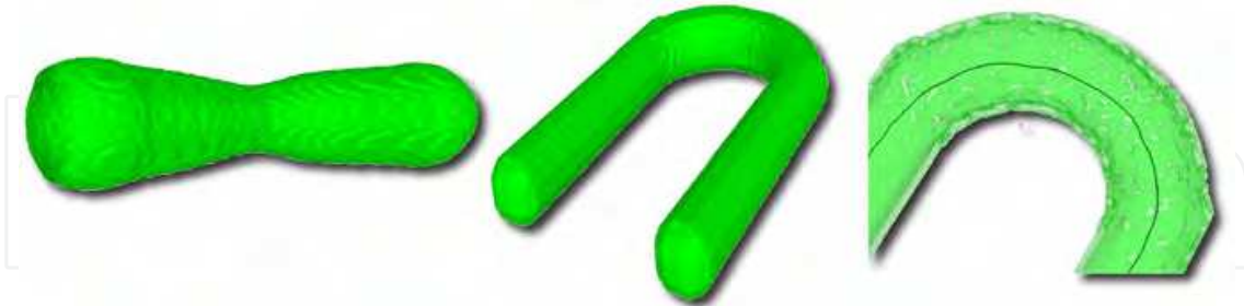
Figure 5. Synthetic environments used for the validation: ( left ) example of straight tube with changing radius; ( center ) u-shaped tube; ( right ) close-up on random noise in u-shaped tube: the central path is also visible
