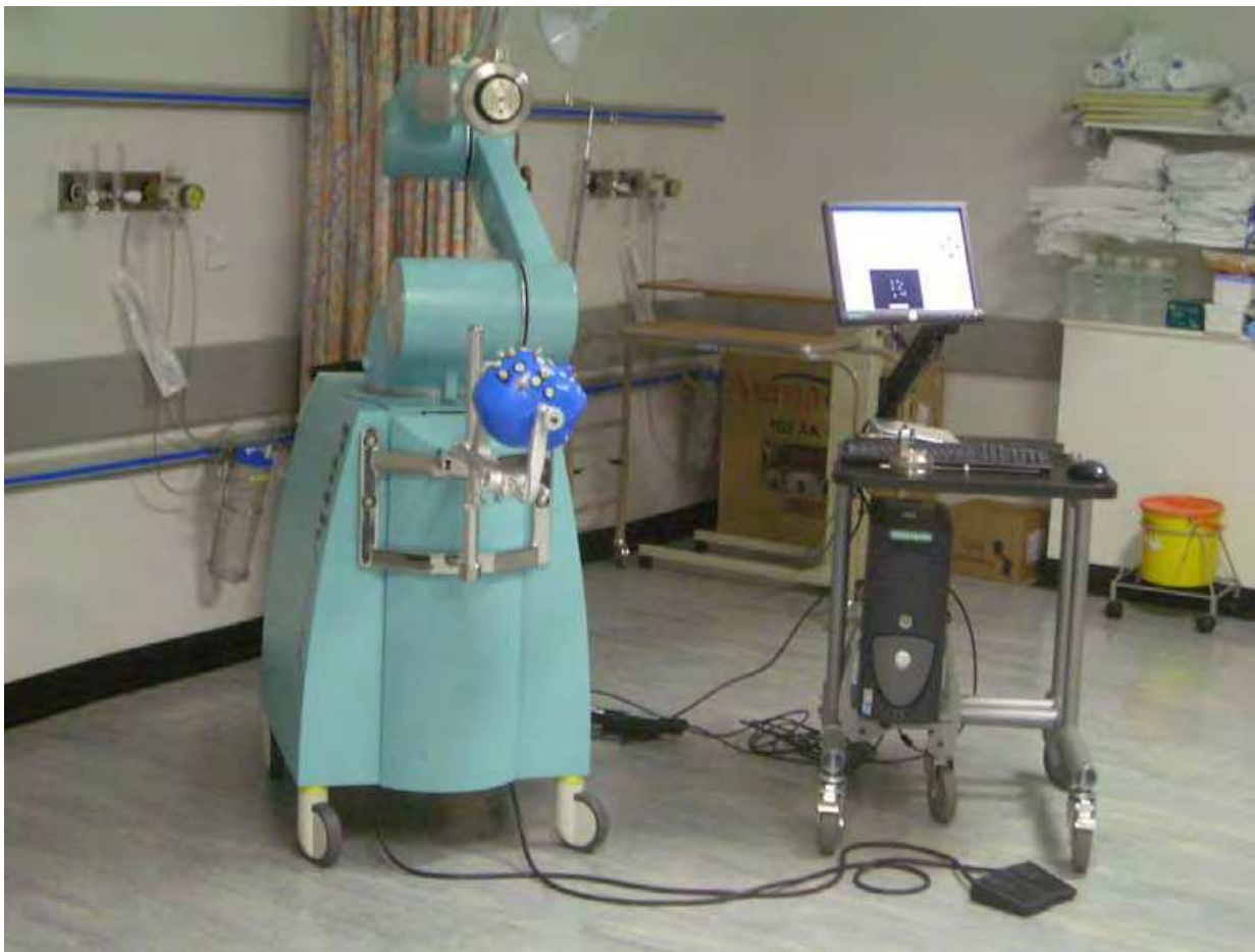
Figure 4. The PathFinder neurosurgical robotic system
