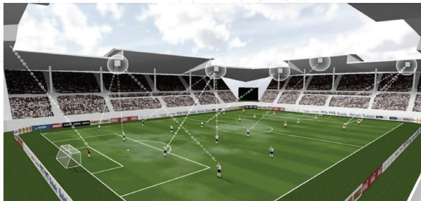
Photo 1. An illustration of the ZXY sports tracking system installed at a football stadium [14].
