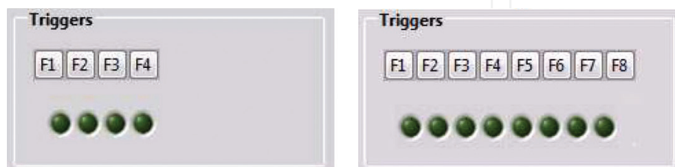
Figure 9. (Courtesy of NIRx Medical Technologies) shows different trigger signals that can be used to set the end and the begging of psycho-physiological stimuli; the marker is set by clicking on the respective button (e.g., F1) or by pushing F1 key on the computer keyboard.
