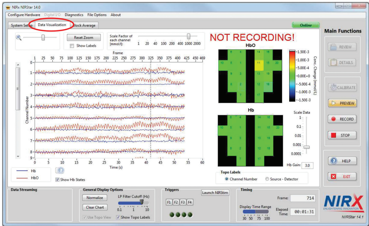
Figure 5. (Courtesy of NIRx Medical Technologies) Data visualization with a trace display on the left side of the screen, topographic layout on the right side of the screen expressing changes in Hb-HbO concentration. Remember that the recorded data are raw data, based on individual wavelengths.
