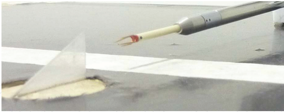
Figure 17. Fin-type vortex generator, with a hot wire anemometer downwards.
